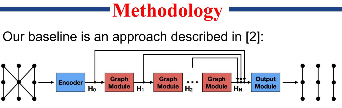
Tracking detector measurements are represented as graph nodes which are associated with one another by learned graph edges that represent the particle tracks
